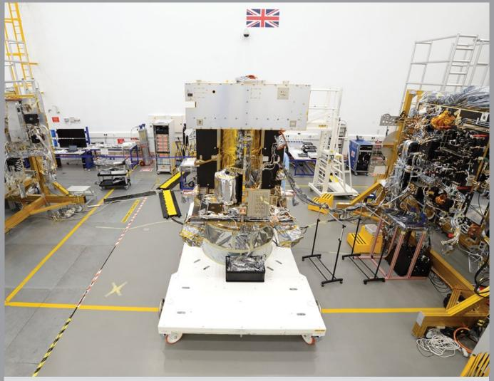
Solar Orbiter core structure (centre), the instrument panel (right) and the spacecraft equipment panels before they were mated together for the first time (Airbus D&S)
